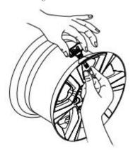
Remove the valve tip cap and nut from the stem, then remove the sensor assembly from the rim.
