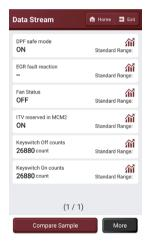
[Compare Sample]: Tap to select the sample DS file. All the values you customized and saved in process of DS sampling will be imported into the Standard Range column for your comparison.
