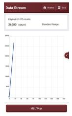
Click [Graph] or [Combine] button and then the system will display the parameters of the selected data streams with wave patterns. If need to remove any items, just deselect them.
