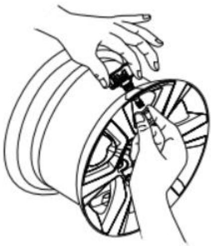
Remove the valve tip cap and nut from the stem, then remove the sensor assembly from the rim.
